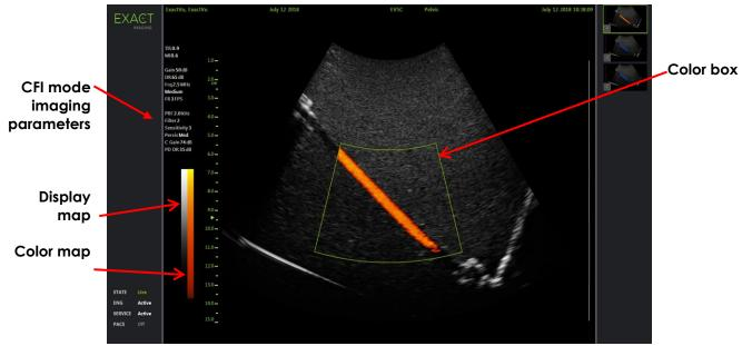
Figure 47: Power Doppler Mode Imaging Screen
