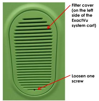
Figure 72: Inside View of Left Side Panel
