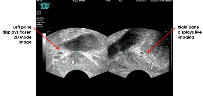
Figure 44: Dual Mode Imaging Screen
