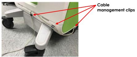
Figure 4: Foot Pedal Cable Management
